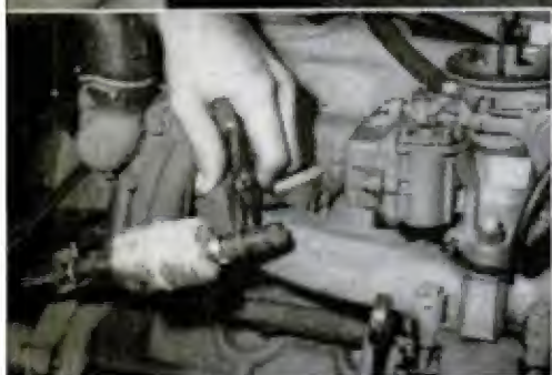
FUEL FILTER , in line to the carburetor, is easily removed for replacement
